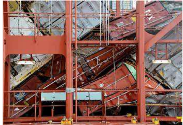
Crushed containers on board MSC Zoe (source DSB).
