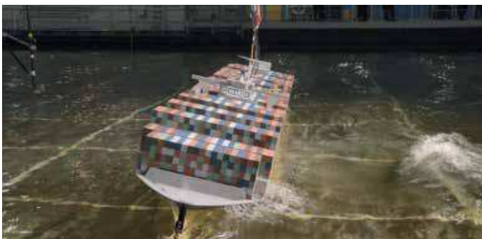
Image of the ship model at the moment of occurrence of a wave impact against the bow and a breaking wave close to the ship (source MARIN).
