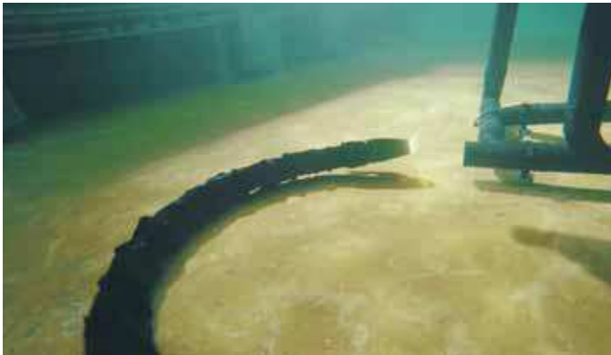
The snake-like underwater robot Eelume can perform planned and on-demand inspections and interventions (by Kongsberg).
