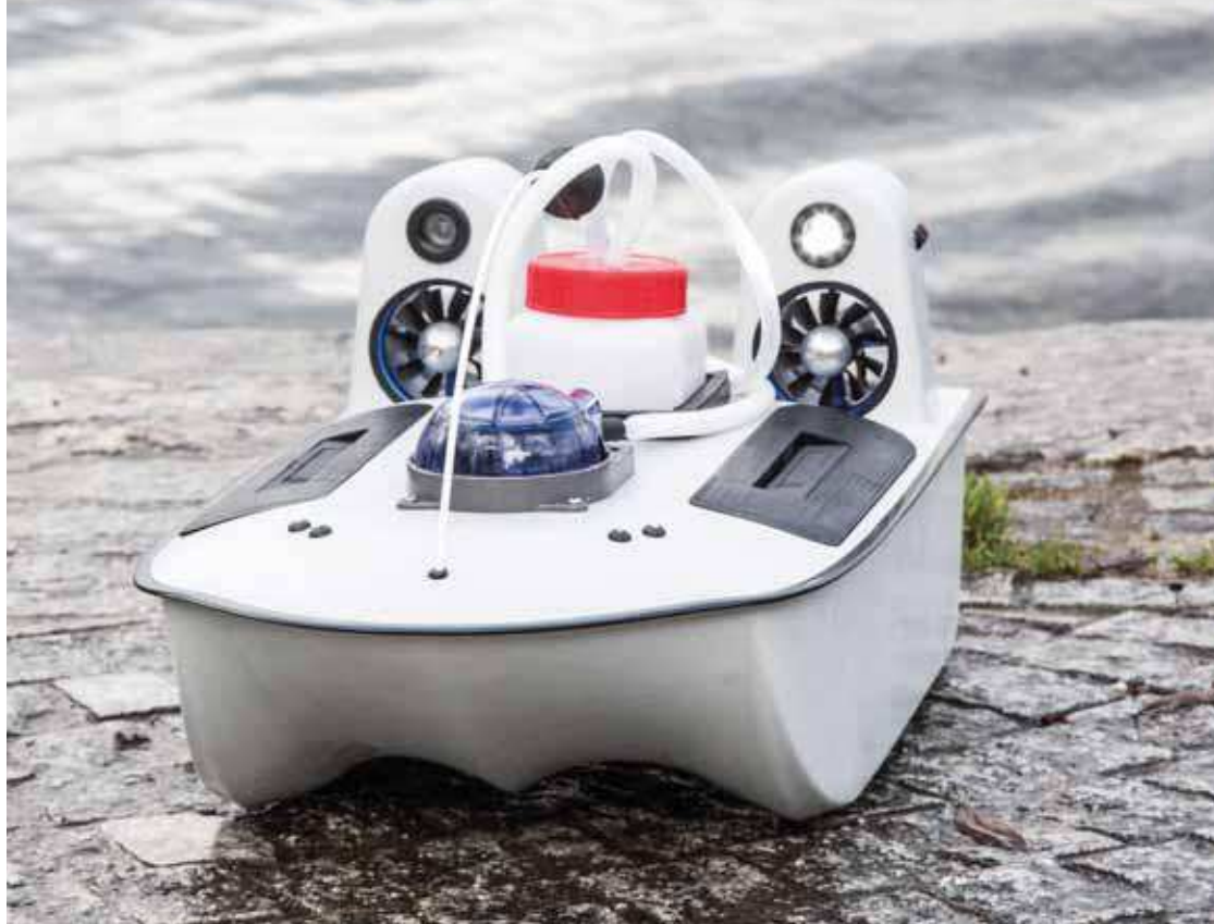
The Spyboat model Duck is a small glassfibre polyester shallow boat propelled by aerial propellers (by Spyboat).
